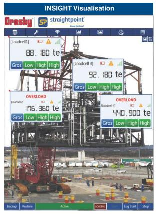
INSIGHT software, supplied with an SW-D USB wireless dongle, allows connection of up to 126 Crosby Straightpoint wireless loadcells simultaneously onto any Windows tablet or laptop.
