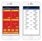
Up to four Crosby Straightpoint, Bluetooth load cells can be connected and monitored by up to eight smartphones, with the HHP2 app installed. It will enable more than one lifting professional to monitor the loads progress and safety, spotting potential dangers or issues from different vantage points.
