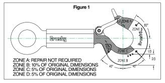
by grinding lengthwise, following the contour of the hook, provided that the reduced dimension is within the limits shown in Figure 1. Contact Crosby Engineering to evaluate any cracks.
