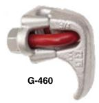
The Bundle Clip is utilized in a choker hitch application to maintain the shape of bundled packages after a load is placed. The Bundle Clip is attached to live line of choker hitch, but it is never to be used as a button or ferrule to carry a load in the primary load path.
