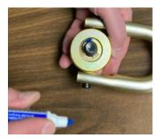
After the inspection, the hoist rings should have an identifier added, that indicates the inspection was performed and found to be acceptable. In this case we placed a blue paint pin dot next to the E-Clip.
