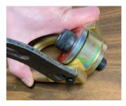
The inspection can be accomplished by taking a small flat rigid object (such as a thin pry bar) that can be inserted under the head of the hinge pin and prying outwardly on the hinge pin.
