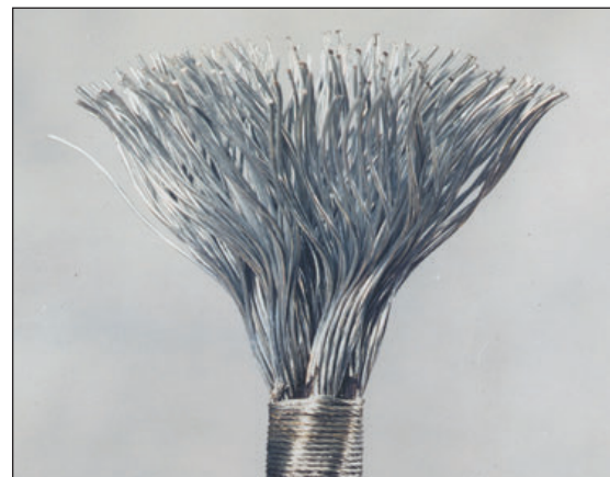
Incorrectly Broomed Wire Rope
