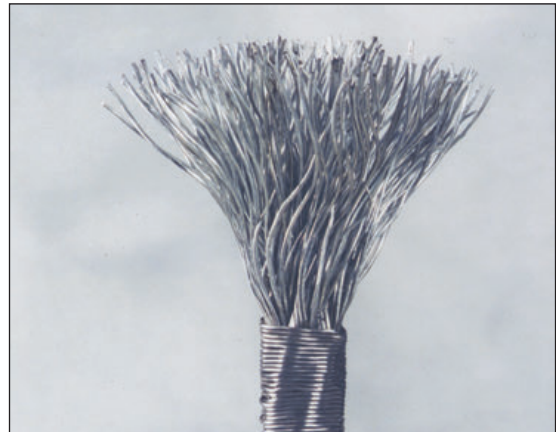
Properly Broomed Wire Rope (Fig. 2)
