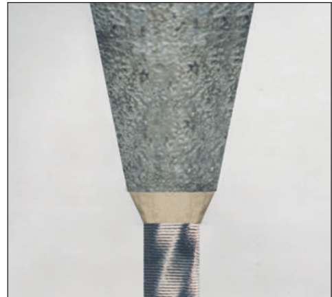
Axes of socket and rope properly aligned and sealed with plasticine (Fig. 4)
