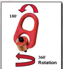
All Crosby swivel style hoist rings are designed and rated to allow full WLL at 90°, and allow bail to pivot 180° with 360° rotation.
