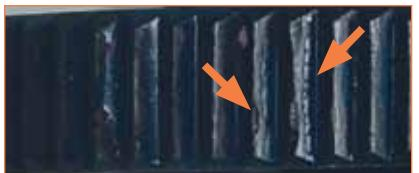
1 complete teeth not sharp and 1 damaged
