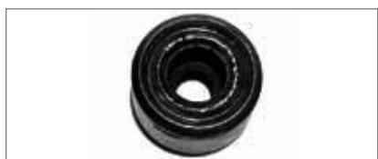
interior ring damaged for 100%
