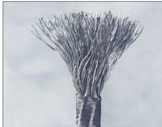
Properly Broomed Wire Rope (Fig. 2)
