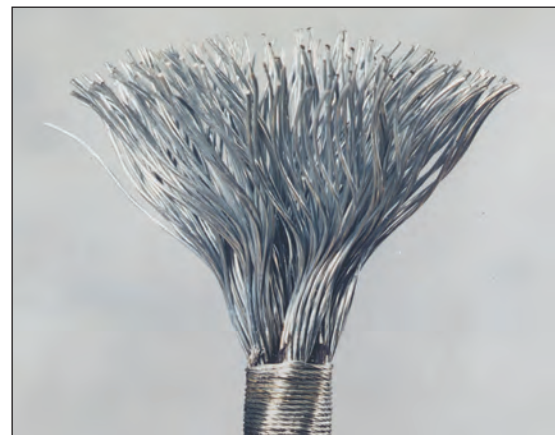
Incorrectly Broomed Wire Rope
