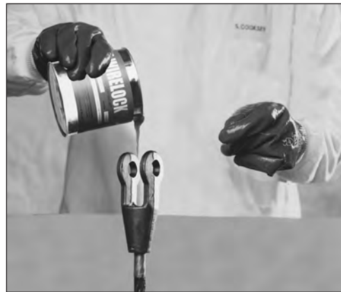
Upon mixing, the compound should be poured immediately (Fig. 7)
