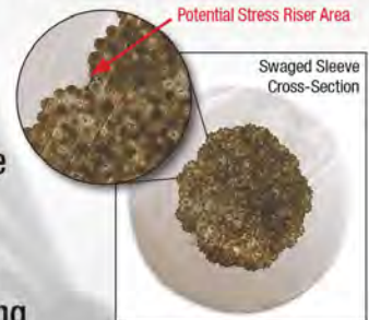
COLD-TUFF® process results in superior ductility that reduces the effects of stress risers.
