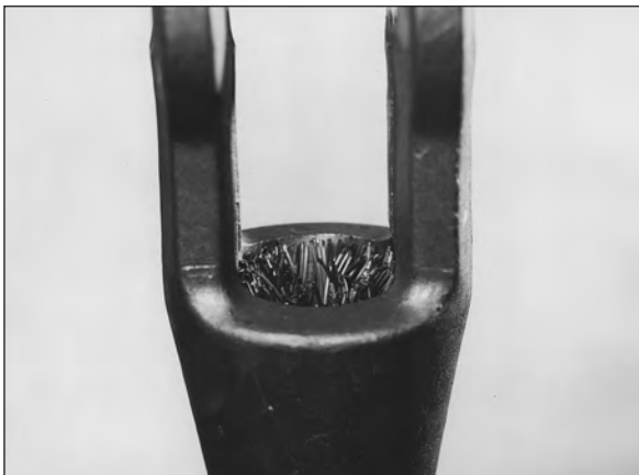
Properly positioned broom with wire rope ends protruding slightly (Fig. 3)
