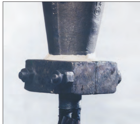
Clamp used to align rope and socket before sealing with plasticine (Fig. 5)
