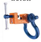
The IPBTO/10 shipbuilding clamp is used as a temporary tackle eye in spaces which have been reinforced with HP (bulb) profiles such as engine rooms and shipsections. This clamp is fitted with a screwed spindle for easy attachment of the clamp. The moment a load is applied, the clamp is automatically fixed.
