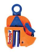
The IPNM10P vertical lifting clamp is used for the lifting, turning, moving or vertical transfer of sheet, plates, or fabrications from horizontal to vertical and down to horizontal (180°) as needed without marring the surface of the material. Materials such as aluminum, stainless steel, painted materials, aircraft skins, composite material, glass, plastic, etc., can be lifted without marring. The protective cover reduces the risk of damage to surrounding plates.
