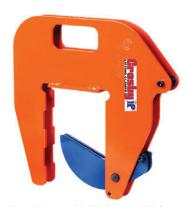
The IPCC is suitable for the vertical lifting and transfer of concrete pipe sections and wells. Very easy application and removal of the clamp thanks to the built-in carrying-grips. Normally used in combination with 7mm chain (not supplied). These clamps must be used in pairs or more.
