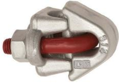
The Bundle Clip is utilized in a choker hitch application to maintain the shape of bundled packages after a load is placed. The Bundle Clip is attached to live line of choker hitch, but it is never to be used as a button or ferrule to carry a load in the primary load path.
