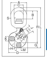
For other swivel hooks designed to rotate under load, see pages 115, 117, 125, 126, 134-137. Use in corrosive environment requires shank and nut inspection in accordance with ASME B30.10-1.10.4 (b)(5)(c) 2009.
